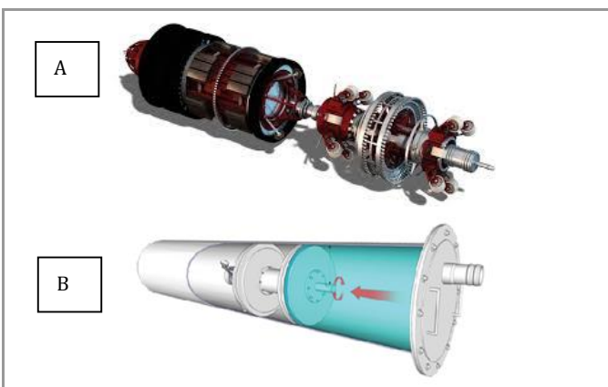
Figure 10. (A) Intelligent Pig, (B) Intelligent Pig moving into pipe launcher [41]
