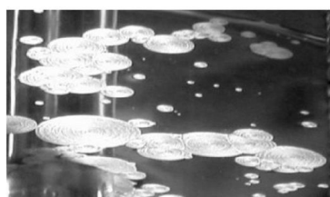
Figure 1. Formation and growth of hydrate crystals at the common water and gas surface
