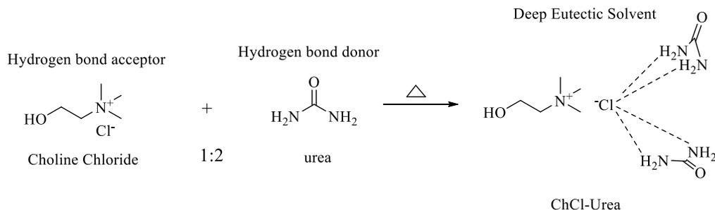
**Figure 3.** A schematic illustration of two component form a deep eutectic solvent (Choline chloride-urea) [29]
