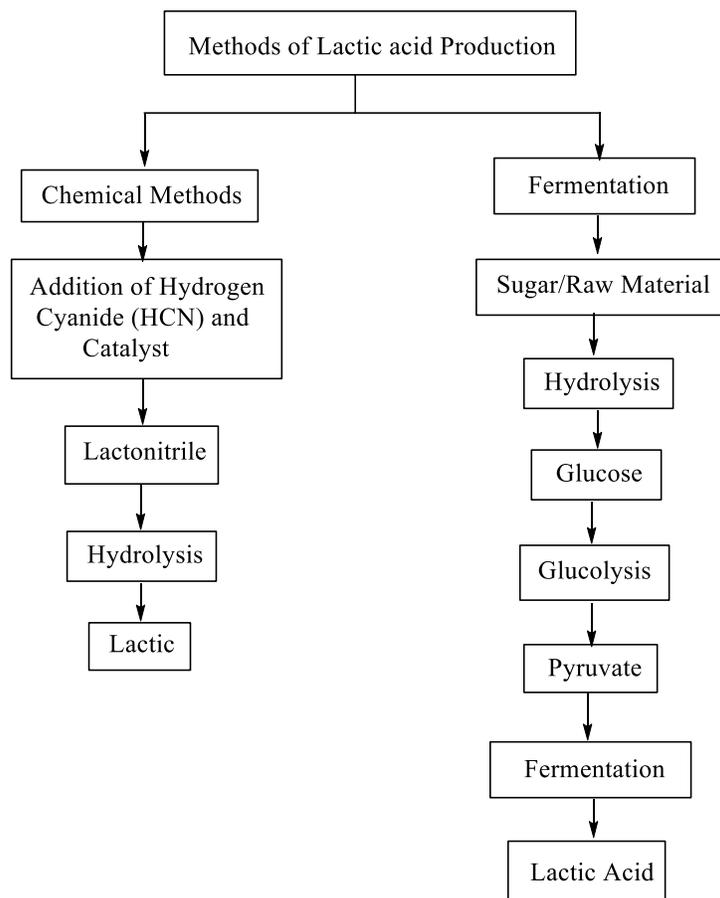
**Figure 4.** Process steps for production of lactic acid via different methods
